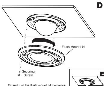
Fit and turn the flush mount lid clockwise onto the base.
