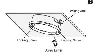
To fasten rotate out the locking arms by turning the screws clockwise.
