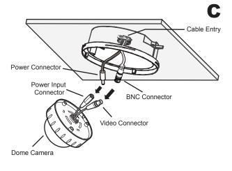
Make the connection to the video and power leads then feed the connectors back through the cable entry; insert the dome onto the threaded portion of the backbox and rotate the dome clockwise to tighten.
