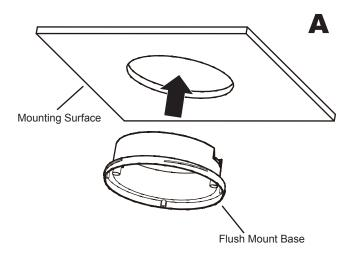
Create an aperture of 5.75 inch (146mm) on the mounting surface to fit the flush mount base.
