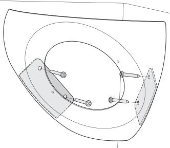
Position the corner mount in the required position. Use screws and wall plugs (as appropriate to the wall surfaces) to fix the corner mount in position. Access to the screw positions is gained through the open front aperture of the corner mount.
