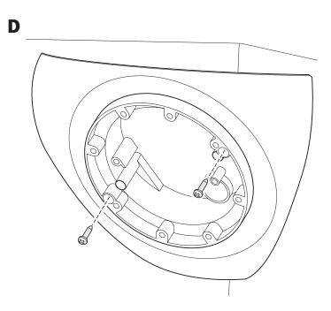
Use the supplied screws to secure the dome enclosure to the corner mount. Continue reassembling, wiring and focussing the dome and its camera according to the supplied instruction sheets.
