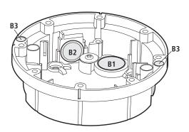
With the camera assembly removed, decide which entry point will be used either (B1) the 3/4" conduit entry or (B2)the 1/2" side conduit entry and remove the appropriate plug. Carefully drill (or tap out) the mounting holes (B3).
