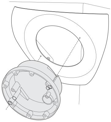
Place the dome enclosure (remove the outer ring, if fitted) within the front aperture of the corner mount. Align the two enclosure mounting holes indicated, with the corresponding threaded holes within the front face of the corner mount.
