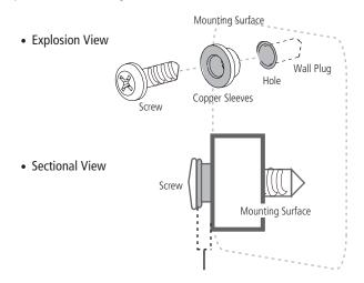
The cooper sleeves create the required space which allows the mount to be installed using the four mounting holes
