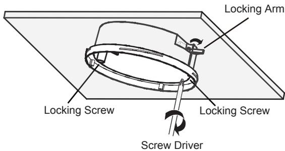
To fasten rotate out the locking arms by turning the screws clockwise.
