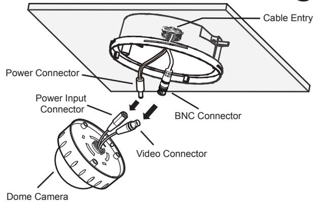
Make the connection to the video and power leads then feed the connectors back through the cable entry; insert the dome onto the threaded portion of the backbox and rotate the dome clockwise to tighten.
