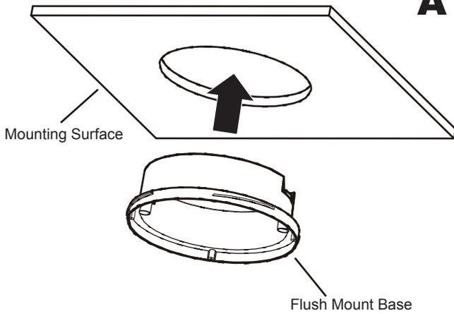
Create an aperture of 5.75 inch (146mm) on the mounting surface to fit the flush mount base.
