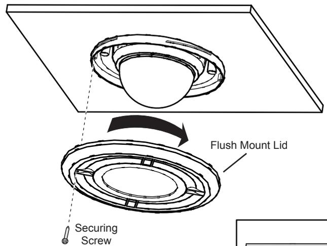
Fit and turn the flush mount lid clockwise onto the base. Insert and tighten the securing screw to complete the installation.
